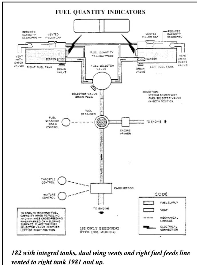
*182 with integral tanks, dual wing vents and right fuel feeds line vented to right tank 1981 and up.*
