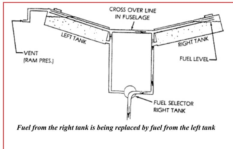
*Fuel from the right tank is being replaced by fuel from the left tank*
