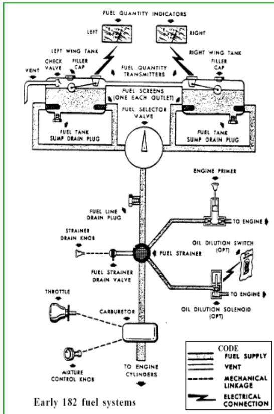
from the left tank. This means that there will not be fuel flow interruption to the engine even if the left tank were to go dry with the fuel selector in the 'BOTH' position.
