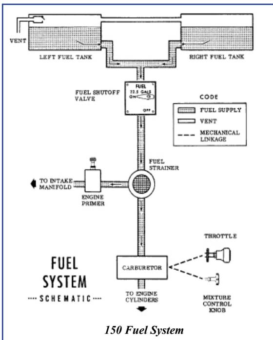
the fuel selector. It is certainly very disconcerting to be flying along and watch your left fuel gauge going down while the right fuel gauge continues to indicate full. The funny thing about this situation is that while only the left gauge is showing fuel usage, the engine may very well be using fuel from the right tank!
